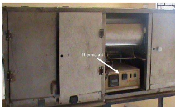
Figure 3.1: The design and constructed metallo-organic chemical vapour deposition (MOCVD) equipment produced by NASENI in collaboration with Prof. E.O.B Ajayi of Physics Department, Obafemi Awolowo University, Ile-Ife.
