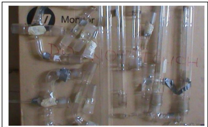
Figure 3.1: The design and constructed metallo-organic chemical vapour deposition (MOCVD) equipment produced by NASENI in collaboration with Prof. E.O.B Ajayi of Physics Department, Obafemi Awolowo University, Ile-Ife.
